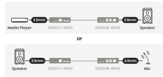
Independent 3.5mm sound channel which can be connected to a microphone or speaker at either Tx or Rx.
