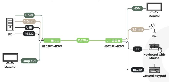
HDMI KVM extension with Audio Input from Rx unit to Audio Output in Tx unit
