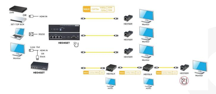
Stack to another HE04SET through HDMI loop out port to get configuration of 1 in 8 out.
