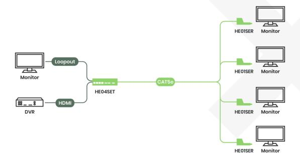
Works with chainable receiver HE01SLR (Max. 3pcs) to get extra transmission distance and outputs.
