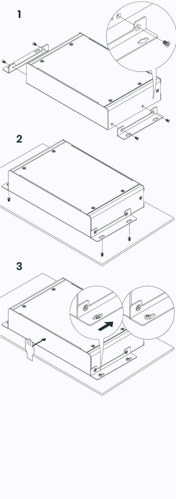
Installed on a Wall
