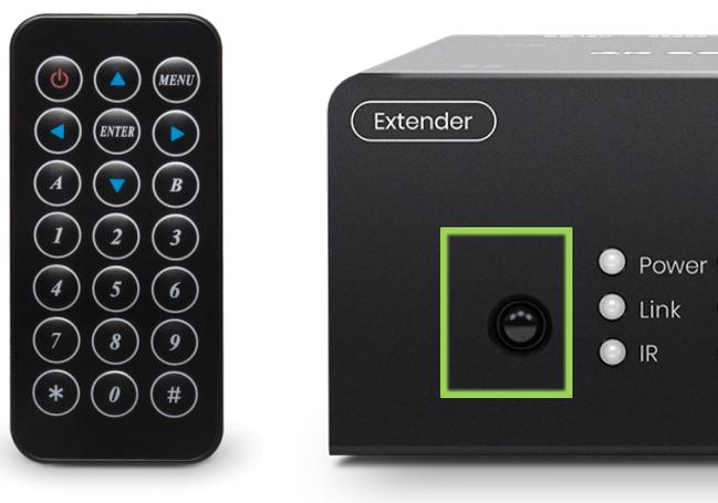
You can use the IR remote for configuration or to switch channels. Simply point the IR Remote at the IR receiver next on the front panel next to the power LED indicator or at the external IR receiver.
